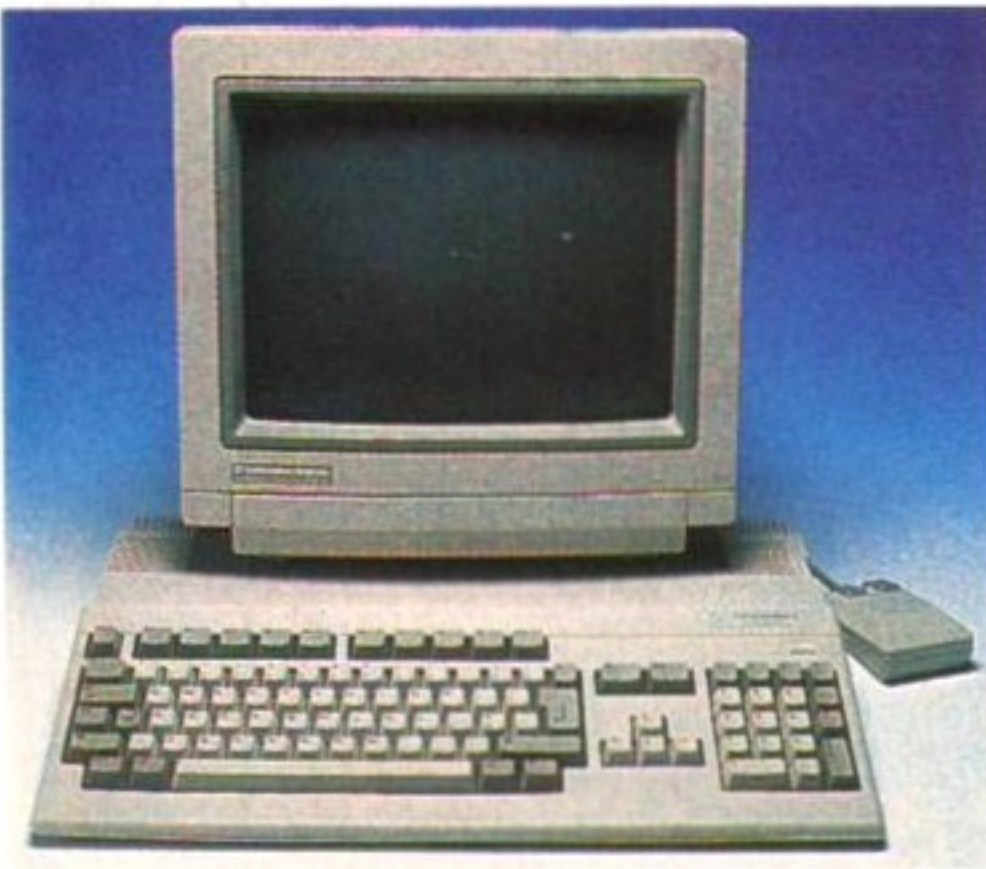
The A500 Plus has the same basic clock circuitry as other Amigas – and badly written software can crash the clock.
