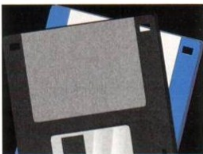
A high density disk is identified by a second hole opposite the protect tab.
